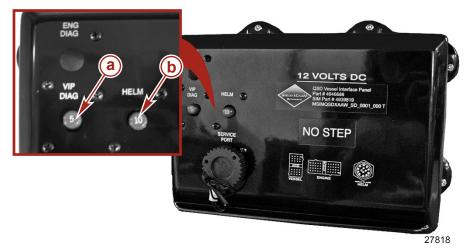
Vessel Integration Panel (VIP) circuit breakers
