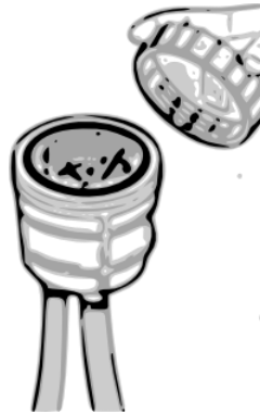
Figure 23 - Sea water filter
