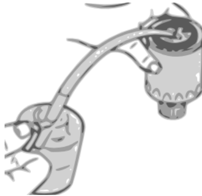
Figure 34 - New oil filter lubrication
