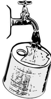
Figure 24 - Sea water filter cleaning under running water
