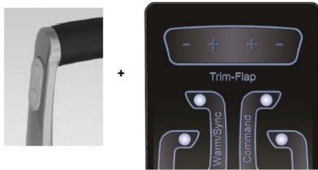
Figure 19 - Trim control for twin engine installation.
