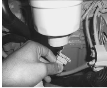
Figure 25 - Removing the water in fuel presence sensor
