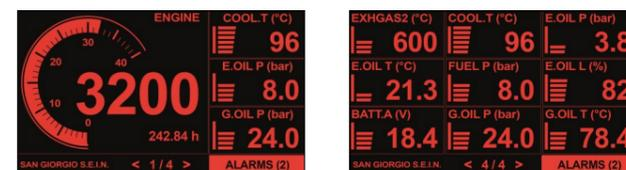
**Night mode** reduces display backlight brightness and draws gauges with black background and red font in order to avoid dazzling and help night vision adaptation.
